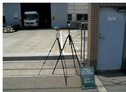
Noise measurement using specialized equipment
